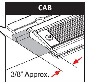
**4** To ensure cover assembly (A) is square for proper operation, make sure attachment holes on the driver and passenger side rails rails (B & C) are lined up across from each other.
