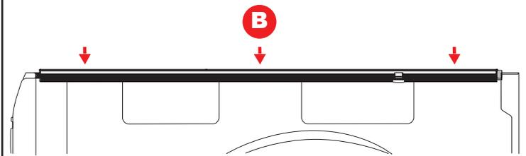
**3** Align drivers side rail (B) so foam is compressed equally on both sides. Compress foam spacer approximately 50%.
