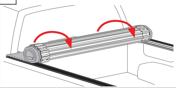
**10** Push down on both ends of the cover (A), near the tailgate, to latch the driver and passenger slam latches. A clicking sound will indicate a correctly installed cover.
